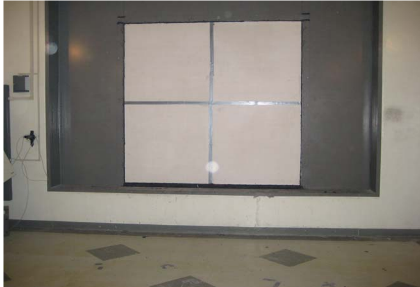
Receive Side of Sample Installed in Test Chamber
