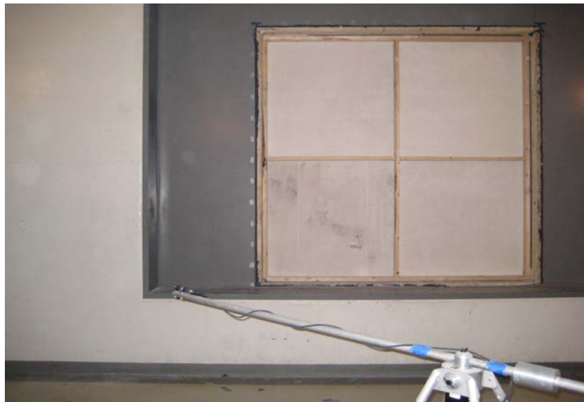
Source Side of Sample Installed in Test Chamber
